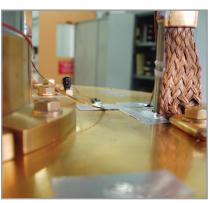
First stage of the 3K cryogen-free cryostat of the Paris-Edinburg pressure cell.
