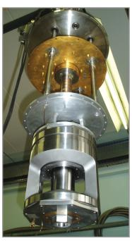
Internal view of the 3K cryogen-free cryostat hosting the Paris-Edinburg pressure cell.
