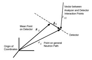
Fig. 2 The relationship between the mean point  $R_d$  on the detector, the general point  $r_d$  and the small deviation of the general point from the mean point,  $\delta_d$ .
