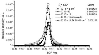
**Fig. 6** Time distributions of neutrons arriving at the detector in the simulated prototype CAS for different sizes of analyzers.
