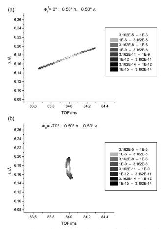
Fig. 5 (a) The distribution of wavelengths as a function of time-ofarrival at the detector, for an unfocused detector oriented normal to the direction of arriving neutrons,  $\phi_d = 0^\circ$  (perpendicular). (b) The distribution of wavelengths as a function of time-of-arrival at the detector, for a detector oriented close to the focused condition,  $\phi_d = 70^\circ \approx \phi_d^f = 69.2^\circ$ .
