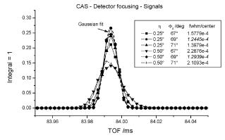
Fig. 4 Time-of-arrival distributions at the detector for a range of detector orientation angles around the focused value,  $\phi_{\rm d}^{\rm f} = 69.2^{\circ}$ .
