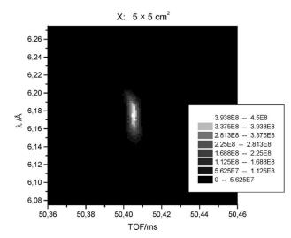
Fig. 8 The distribution of wavelengths and time-of-arrival for focused conditions.
