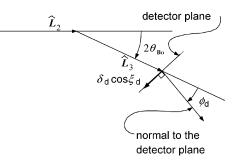
Fig. 3 The detector illustrated in the "analysis plane" defined by vectors  $L_2$  and  $L_3$ . The focused detector orientation is perpendicular to the analysis plane.
