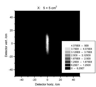
Fig. 9 The distribution of neutrons in the vertical and horizontal directions on the detector for focused conditions.
