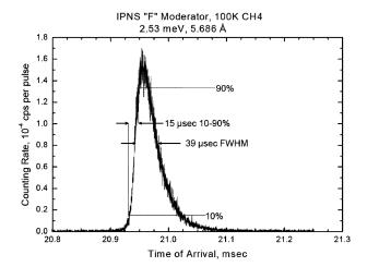
Fig. 10 The emission-time distribution of the IPNS "F" moderator for 5.7 Å neutrons. The time scale is offset according to the arrival time of the neutrons at 11.7 m distance. The 10–90% rise time is 15  $\mu$ s. The FWHM is 39  $\mu$ s.
