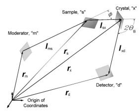
Fig. 1 Schematic diagram of the pulsed-source crystal analyzer. The lines represent a general path through the instrument.  $I_{xd} = R_d - R_x + \delta_d - \delta_x = L_{xd} + \delta_d - \delta_x$ .
