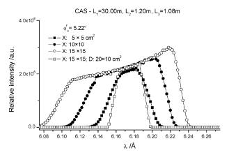
**Fig. 7** The distributions of wavelengths accepted by the instrument as functions of the size of the analyzer crystal.
