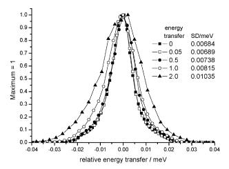
**Fig. 11** The change in energy resolution at various energy transfers keeping the same focusing condition obtained for elastic scattering.
