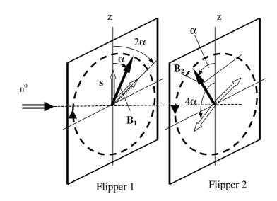
Fig. 7.17 The bootstrap configuration consist of two closely placed spin flippers with magnetic fields rotating in opposite direction. Open arrows are neutron spin positions. Black arrows are rotating magnetic fields.
