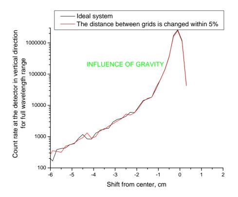
Fig. 5.13 Count rate in vertical direction at the PSD detector.
