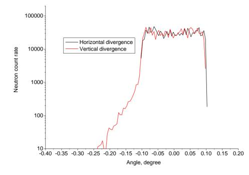
Fig. 5.16 The intensity as a function of vertical and horizontal divergence at the exit of the grid system for the whole wavelength band for a sample sizes  $4x4cm^2$ .
