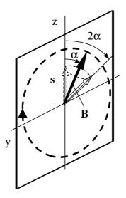
Fig. 7.1 The spin flipper with the rotating magnetic field. Rotation of the neutron spin vector is performed by Larmor precession of the neutron spin by the angle  $\pi$  around the magnetic field vector **B**, as (6.3) equation is required. The angle  $\alpha$  is an initial phase of the rotating magnetic field. Initial position of the neutron spin is directed vertically upward (parallel to the axis Z).
