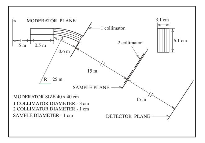
Fig. 5.9 Example of a SANS instrument with classical pinhole collimation [55].
