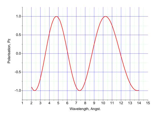
Fig. 6.9. Monte Carlo simulations: wavelength dependence of the polarisation at the exit of an RF flipper.
