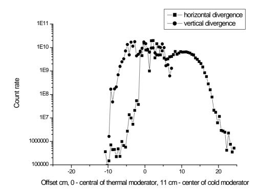
Fig. 5.2 The acceptance of the "multi-spectral" extraction system in both directions. The diameter of the cold moderator is 15 cm and center is shitted 11 cm relative to the origin in the right side. The size of the thermal moderator is  $60x60 \text{ cm}^2$ . The thermal moderator is centered.
