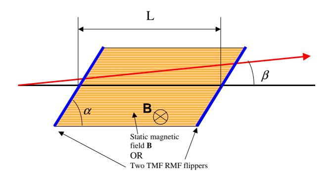
Fig. 7.10 One (first or second) arm of the SESANS instrument in the case of a classical spin echo setup and a TMF RMF spin echo. The red arrow is a neutron path. Two TMF RMF flippers can be installed instead a magnetic field region, but these flippers and the static magnetic field *cannot* be used together! The precession angle  $\varphi$  can be calculated by the formula (7.1) multiplying by the additional factor (1/sin( $\alpha$ )).
