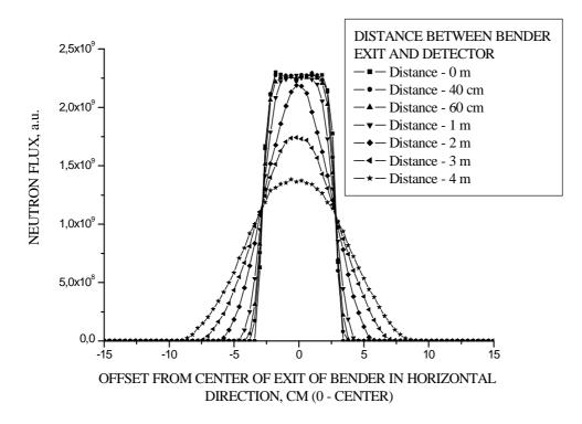
Fig. 4.9 Neutron flux profile for bender 3 of table 4.2.
