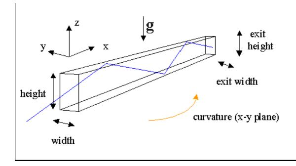
Fig. 4.1 Neutron guide, general example.
