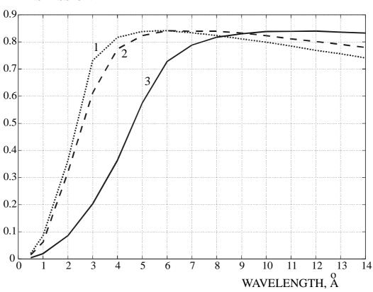
Fig. 4.3 Line 1 (dots) – transmission of the supermirror bender (m=2). Line 2 (dashed) – transmission of the natural nickel-coated guide. Line 3 – transmission of the bender with a natural nickel coating [55].
