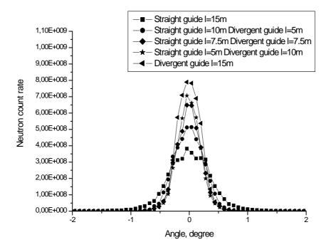
Fig. 5.6. The vertical divergence at the exit of guide for all wavelength band: 1...20 Å.
