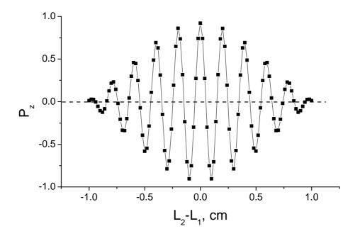
Fig. 7.6 NSE signal obtained for f = 50 kHz and  $L_1 = L_2 = 1$  m. Neutron wavelength  $\lambda_0 = 20$  Å ( $\Delta\lambda/\lambda_0 = 20\%$ ).
