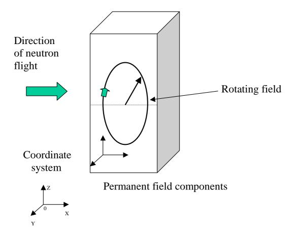
Fig. 3.5 Rotating and permanent magnetic fields configuration. Small green arrow is direction of rotation of a magnetic field.
