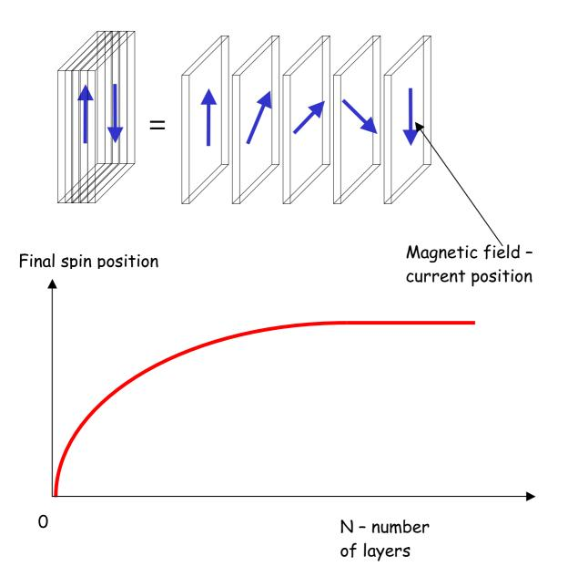
Fig. 3.6 Dividing the precession volume into a number of layers. Blue arrows are current directions of a rotating magnetic field. Dependence of the final spin position on the number of slices N.
