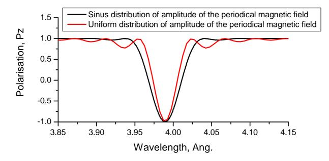
Fig. 3.8 Simulations of the "Drabkin resonator" for two kinds of amplitude distribution of the periodical magnetic field: final distribution  $P_z(\lambda)$ . Initial polarisation of a incident beam is  $P_z=1$ . Final polarisation is -1 only for the resonance wavelength  $\approx 4$  Å.
