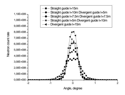
Fig. 5.5. The beam intensity as a function of the horizontal divergence at the exit of the guide for all wavelength band: 1...20 Å.
