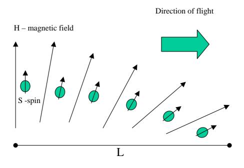
Fig. 6.5 The polarisation follows the direction of the magnetic field adiabatically for slowly varying magnetic field H.
