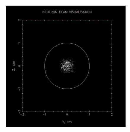
Fig. 5.12 Direct beam at a PSD detector without gravity for multi pinhole collimation system.
