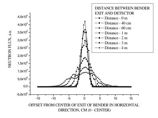
Fig. 4.10 Neutron flux profile for bender 2 of table 4.2.
