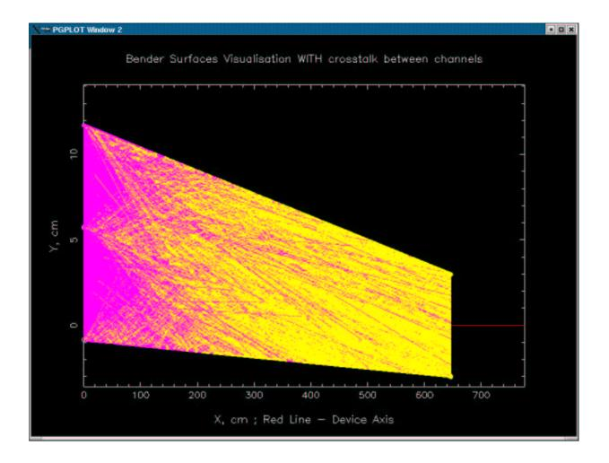
Fig. 5.3 Visualisation of neutron paths in the beam extraction system. The yellow lines show trajectories after the first reflection, the neutrons fly from the left to the right emerging from the thermal (lower part) and the cold (upper part) moderator.
