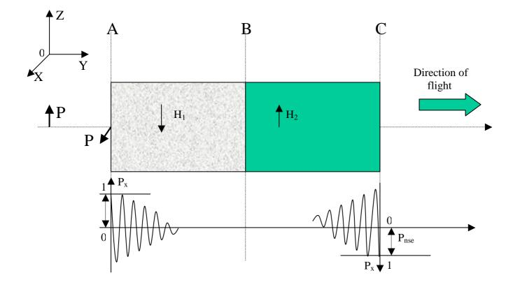
Fig. 6.7 General layout of a neutron spin echo spectrometer.
