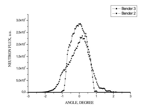
Fig. 4.11 Vertical divergence for the bender 2 and 3 of table 4.2.
