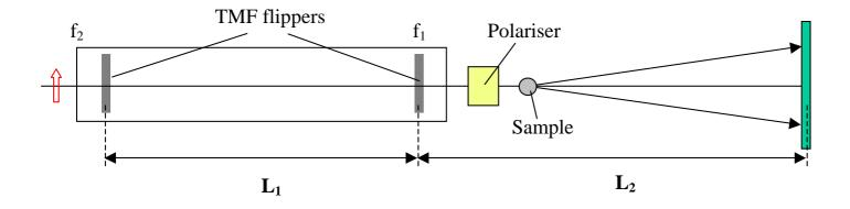
Fig. 7.15 General layout of a MIEZE instrument. The red arrow is initial position of neutron spin.
