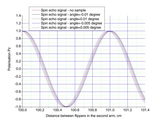
Fig. 7.12 Shift of the NSE signals caused by the deviation angles  $\beta=\pm 0.01^{\circ}$ and  $\beta=\pm 0.005^{\circ}$  of a practically uncollimated (± 1°) neutron beam in horizontal plane for the RMF flipper's driving frequency of  $f_B=50$ kHz, the distance between foils in the first arm is L=1m and the inclination angle of all foils is  $\alpha=45^{\circ}$ . Thickness of all flippers is 0.0025 cm. Incident wavelength band is 3.98 ... 4.02 Å.
