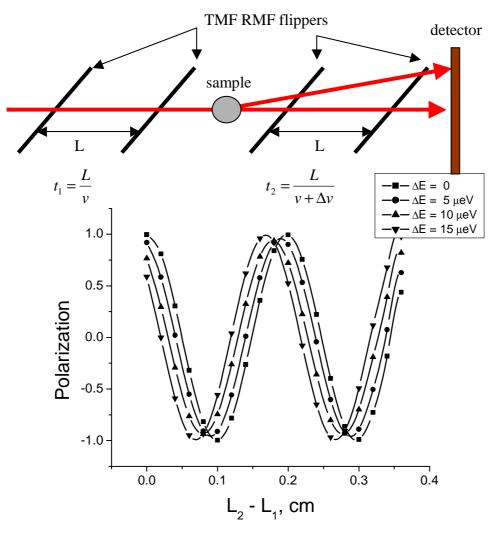
Fig. 7.8 NSE setup for inelastic scattering. The shift of NSE signal corresponding to the energy exchange  $\Delta E \approx \Delta v$  on the sample. The v is the neutron velocity,  $\Delta v$  is velocity changing of a neutron on the sample. Monte Carlo simulations were carried out for TMF spin flippers (f = 250 kHz)
