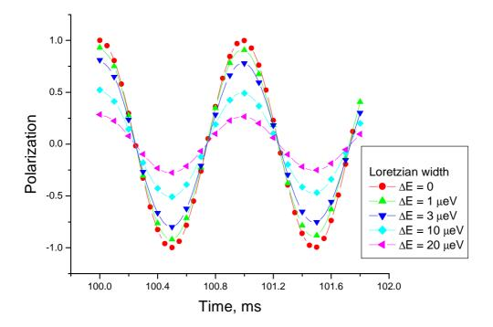
Fig. 7.16 MIEZE instrument simulations: red line – no sample, other lines a quasielastic sample with the Loretzian model [42].
