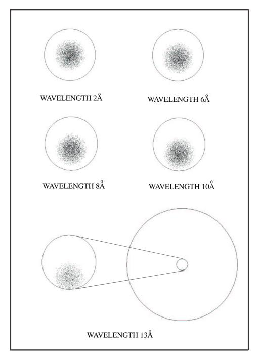
Fig. 5.10. The direct neutron beam at the detector. The diameter of the small circle is 8 cm and the diameter of the big circle – is 80 cm. [55]
