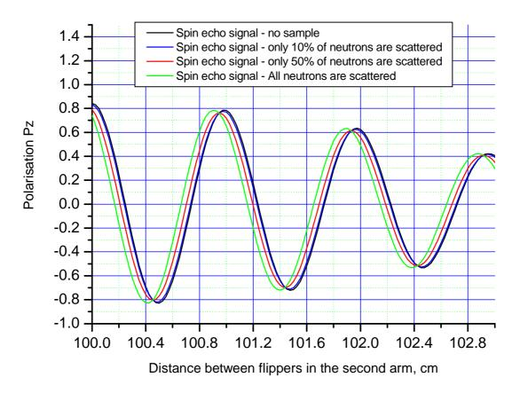
Fig. 7.14 Shift with amplitude degradation of the NSE signals caused by the deviation angles of a practically uncollimated ( $\pm$  1°) neutron beam in horizontal plane for three kinds of samples, described before. The inclination angle of all foils is  $\alpha$ =15°. Thickness of all flippers is 0.0025 cm. The deviation angle is  $\beta$ =0.01°.
