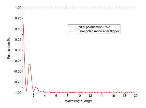
Fig. 3.10. Flipping of a polarised neutron beam by the gradient flipper: final distribution  $P_z(\lambda)$ . Initial polarisation of an incident beam is  $P_z=1$ .
