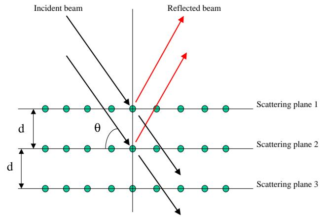
Fig. 2.2 Bragg's diffraction of neutrons, electrons or x-rays. The incident beam should be non-monochromatic to simplify the satisfaction of all parameters in Bragg law (2.8) during the experiments but in general a monochromatic beam is acceptable as well.
