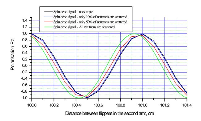
Fig. 7.13 Shift with amplitude degradation of the NSE signals caused by the deviation angles of a practically uncollimated ( $\pm$  1°) neutron beam in horizontal plane for three kinds of samples, described before. The inclination angle of all foils is  $\alpha$ =15°. Thickness of all flippers is 0.0025 cm. The deviation angle is  $\beta$ =0.01°. Incident wavelength band is 3.98 ... 4.02 Å.
