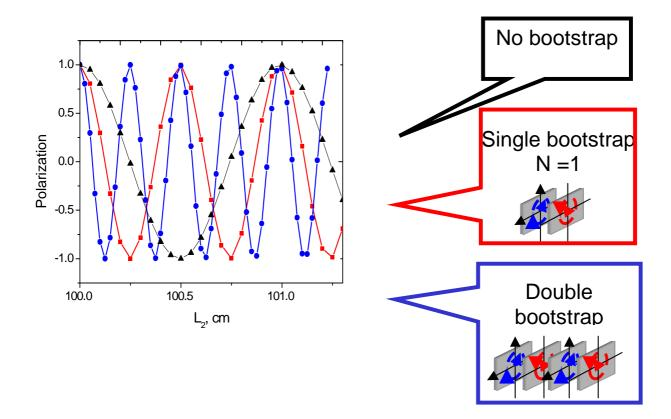
Fig. 7.18 Bootstrap: simulated NSE signal for three instruments.
