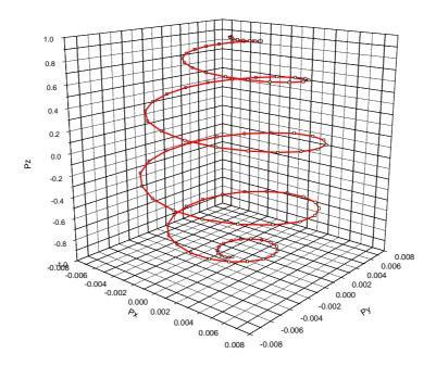
Fig. 6.11 The motion or evolution of the neutron spin in the flipper. Initial point  $S_i=(0,0,1)$  and final point  $S_f=(0,0,-1)$ .
