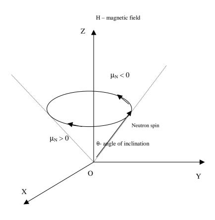
Fig. 6.1 Precession of a neutron spin around the magnetic field **H** and directions of precession for different signs of  $\mu_{N}$ .
