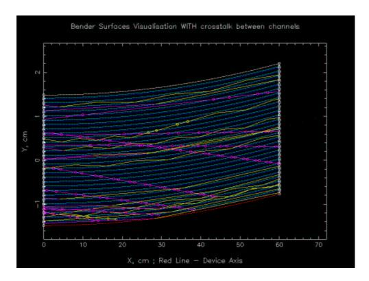
Fig. 4.5 Normal (classical) bender during simulations with neutron flight paths.
