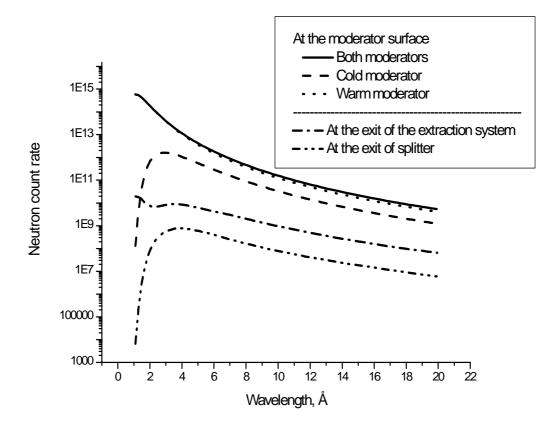
Fig. 5.4 The count rate at the moderator surface, exit of the extraction system and exit of the splitter for the VSANS beam line. Neutron count rate at the exit of the extraction system proves the efficient performance of the presented beam extraction system: sum of two Maxwell distributions.
