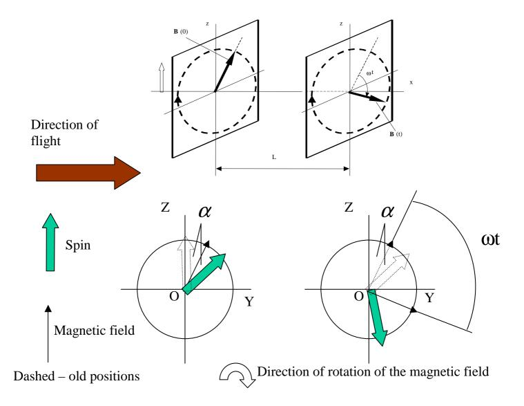
Fig. 7.4 Pair of thin magnetic field flippers. Demonstration of the independence of the total precession angle  $\varphi$  (see formula (7.4)) from the arrival time of flight of a neutron at the first flipper foil or the initial phase  $\alpha$  of the rotating magnetic field.
