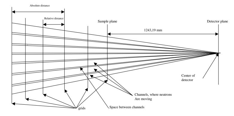
The proposed collimation system for VSANS will have a "multi converging apertures" structure [5, 58], see figure 5.11.
