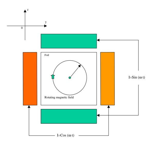
Fig. 7.3 General scheme for producing the rotating magnetic field in a foil.
