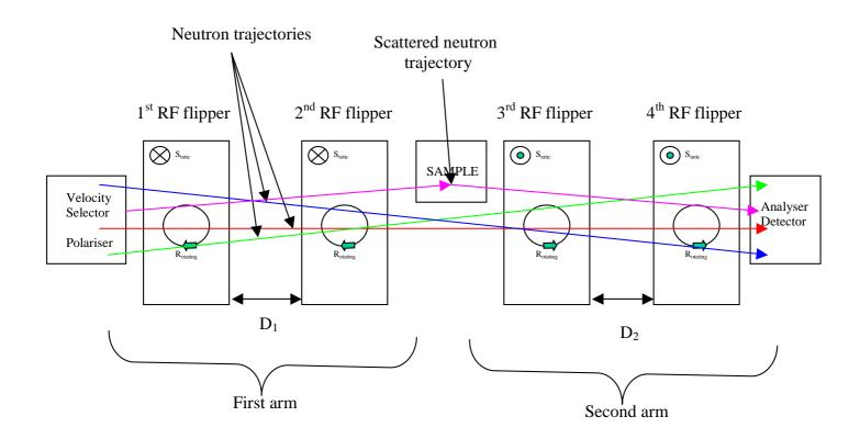
Fig. 6.12 General neutron resonance spin echo spectrometer (NRSE). Between RF flippers in the each arm, there is no magnetic field as well as in the sample area.
