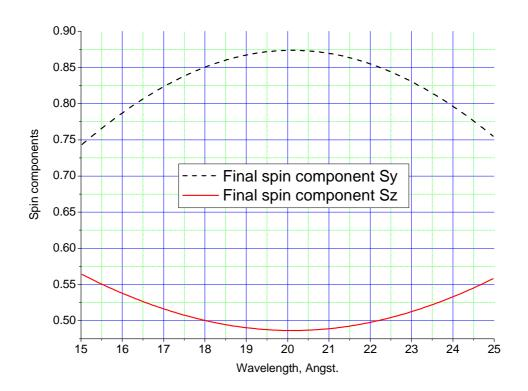
Fig. 7.2 The simulation of the thin magnetic field spin flipper with the rotating magnetic field. Amplitude of rotating magnetic field is 3391.19 Oe, frequency is 50 kHz, initial phase  $\alpha$ =30 degree. Thickness of the foil is 0.001 cm, the number of layers is 40 along the direction of propagation. The flipper has been adjusted for a wavelength  $\lambda$ ≈20Å. The expected spin components for this wavelength: S<sub>Y</sub>=0.866, S<sub>Z</sub>=0.5 for the instant magnetic field.
