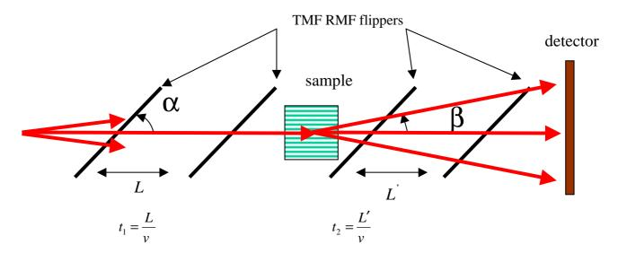
Fig. 7.9 SESANS or SERGIS (collimation only in the horizontal direction) configurations. The angle  $\alpha$  is an angle of a foil inclination. The angle  $\beta$  is angle of scattering in a sample. It is assumed only elastic scattering without the energy changing. The  $\nu$  is the velocity of a neutron.
