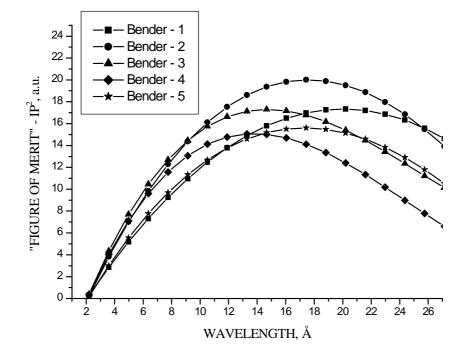
Fig. 4.7 The wavelength dependence of the "figure of merit" for benders from table 4.2 with a radius of curvature of 1500 cm.
