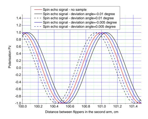
Fig. 7.11 Shift of the NSE signals caused by the deviation angles  $\beta=\pm 0.01^{\circ}$ and  $\beta=\pm 0.005^{\circ}$  of a practically uncollimated ( $\pm 1^{\circ}$ ) neutron beam in horizontal plane for the RMF flipper's driving frequency of  $f_B=50$ kHz, the distance between foils in the first arm is L=1m and the inclination angle of all foils is  $\alpha=15^{\circ}$ . Thickness of all flippers is 0.0025 cm. Incident wavelength band is 3.98 ... 4.02 Å.
