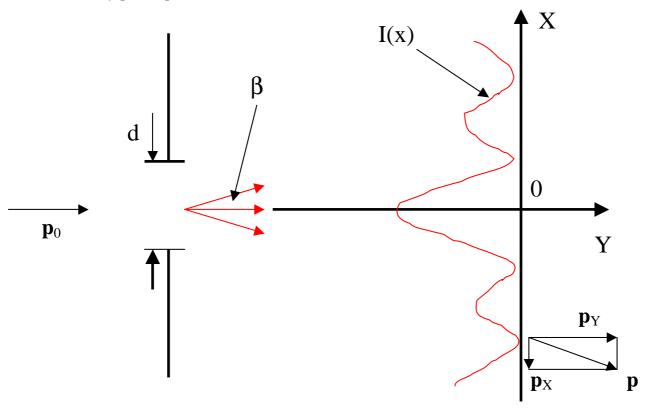
Fig. 2.1 Diffraction of a particle with initial momentum  $\mathbf{p}_0$  at a slit [87]. Note, that a particle has wave properties according De Broglie equation (2.1). The De Broglie wavelength  $\lambda_{DB}$  of a particle has to be comparable to the size of
