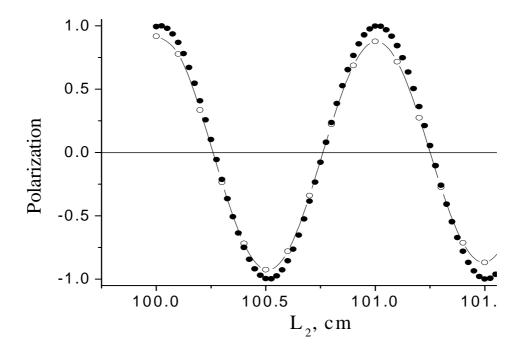
Fig. 7.7 Degradation of the NSE signal (open circles) for random deviations within 5% of the foil thickness for all four TMF spin flippers in the NSE
