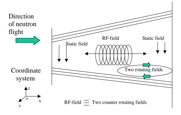
Fig. 3.9 Gradient flipper: field configurations. Initial spin position is parallel to the axis OZ and directed vertically upward.
