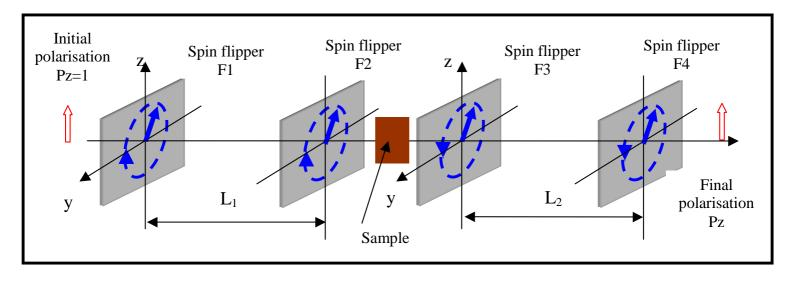
Fig. 7.5 General layout of the neutron spin echo spectrometer consisting of two pairs of the thin magnetic foils flippers with rotating fields.
